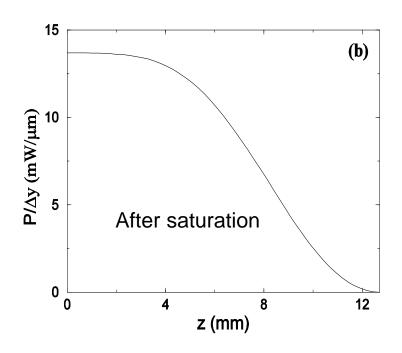
For  $I/\Delta y = 50$  A/m, at saturation,  $P/\Delta y = 13.7$  mW/ $\mu$ m Power e-folding time = 0.2 ns (simulation) 0.17 ns (analytic formula)
